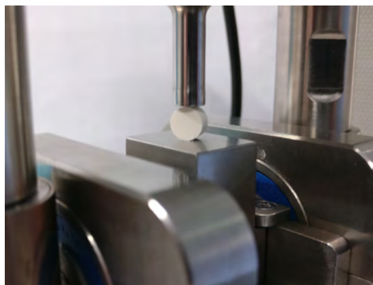
Figure 3: Tensile strength testing of a manufactured tablet.
